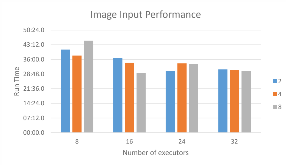
Figure 3: Image import performance, varying the number of executors on the cluster and RAM per executor
