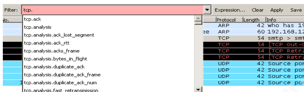
Figure 4: Wireshark auto-lookup feature, listing valid protocol field names.
