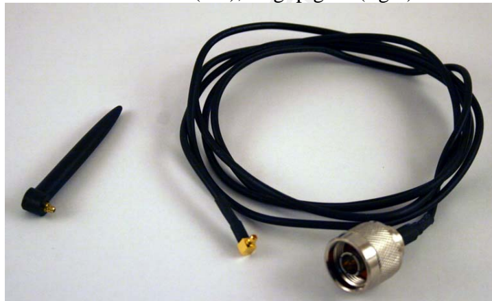
Figure 17 – Omnidirectional Antenna (left), Yagi pigtail (right)
