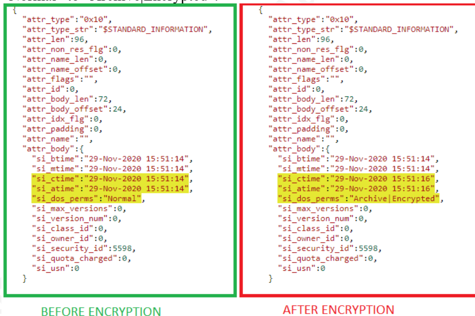
Figure 5-1: The MFT STANDARD_INFORMATION attribute of a file before/after encryption
