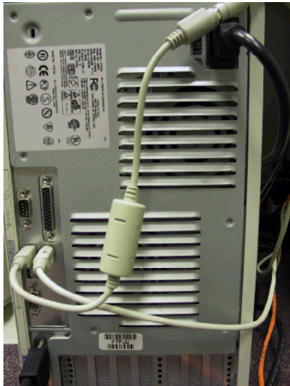
Keyboard cable with KeyGhost installed
