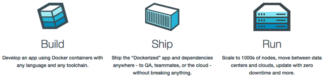
Figure 3: Docker build-ship-run workflow (Knoll 2018)
