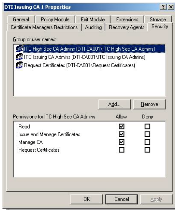
Figure 3-12: The permissions set by the CA administrators on the issuing CAs. The groups are local groups on each CA to which domain global groups have been added.
