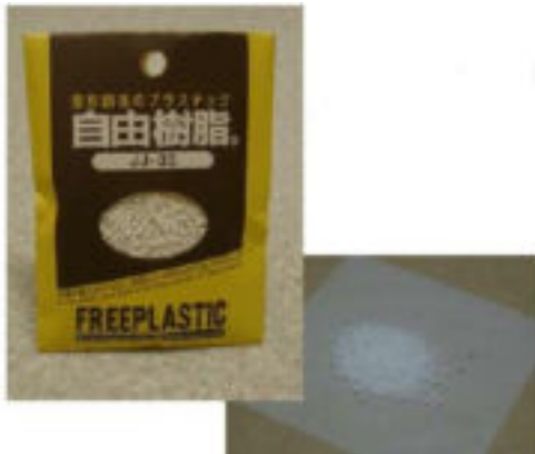
Fig. 2. Freeplastic used for fingerprint mold
