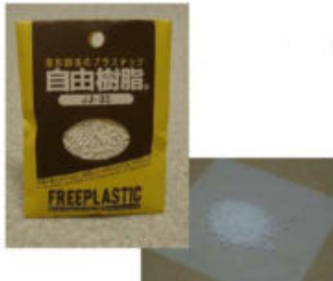
Fig. 2. Freeplastic used for fingerprint mold
