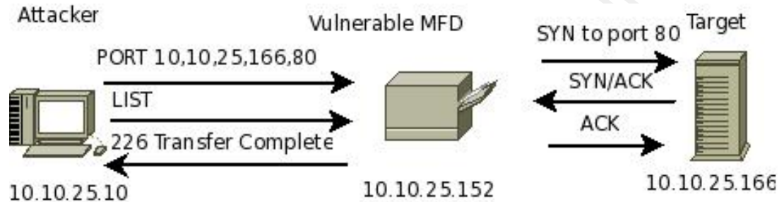
Figure 1: An illustration of the FTP bounce attack (adapted from Messer, 2007).
